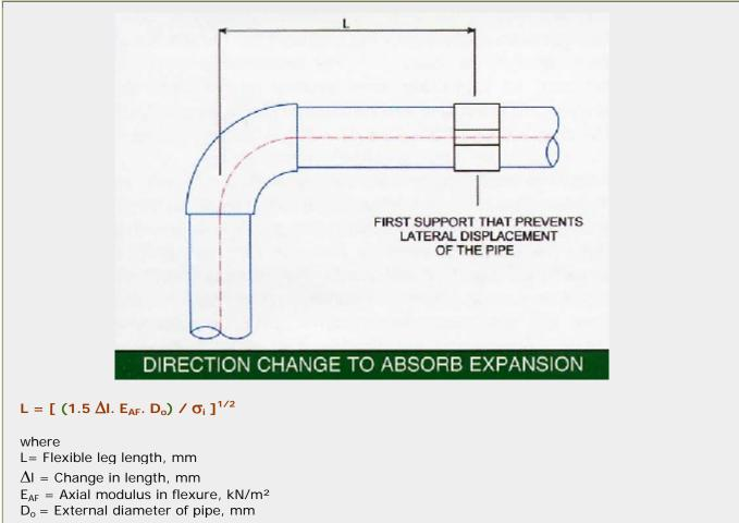
$\sigma_i$  = Remaining axial stress, kN/m<sup>2</sup>
